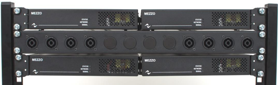
This picture illustrates a typical 16-channel KET hardware rack equipped with 4 Mezzo 4-channel power amplifiers and one optional Ket Mezzo Patch-Bay.
