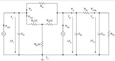
The heating of the voice coil is modeled by a nonlinear thermal equivalent circuit. The model describes the heat transfer from the voice coil to the pole tips and the magnet. It considers convection cooling (dependent on cone displacement and velocity) and direct heating of voice coil and magnet due to eddy currents.
