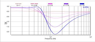
DC component in the voice coil generated dynamically by a sinusoidal tone.
