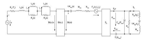
The lumped-parameter model shown above is used to describe the large signal behavior of electro-dynamical transducers mounted in common acoustical systems (sealed or vented enclosure, passive radiator, bandpass). In contrast to the well-known linear model the components of the large signal model are not constant but rather depend on one or more speaker states (like displacement x, voice coil temperature  $T_v$ , sound pressure  $p_{box}$ , or volume velocity  $q_p$  in the port).
