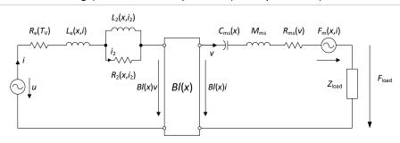
The lumped-parameter model shown above is used to describe the large signal behavior of electro-dynamical drivers at high amplitudes. In contrast to the well-known linear model the elements
