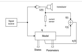
The transducer model is implemented as an adaptive system in a digital signal processor (DSP). The transducer is persistently excited by a broadband noise or multi-tone signal generated by a signal source via a power amplifier. The model which is excited with the voltage U(t) estimates the voice coil current I(t) which is then compared with the measured current I(t). The amplitude of the difference signal (error) is minimized by adjust-
