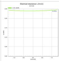
The nonlinear B(H) characteristic of the iron causes a variation of the inductance L(i) versus voice coil current i. This nonlinearity is also called flux modulation or better permeability modulation. A symmetric characteristic shows a saturation of the iron at high positive and negative current. The curve becomes asymmetric for a high DC flux generated by the magnet. The parameter L(i) causes harmonic distortion at higher frequencies which can easily be detected in the input current.
