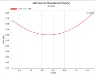
The dependency of the mechanical resistance  $R_{\rm ms}$  on voice coil velocity v is a dominant nonlinearity in micro-speakers and other transducers which have a relatively high resonance frequency  $f_{\rm s}$ , a relatively small force factor Bl and a total quality factor  $Q_{\rm ts}$  dominated by the mechanical losses. The  $R_{\rm ms}(v)$  nonlinearity causes a significant increase of the mechanical damping at resonance frequency, causing a nonlinear ampli-
