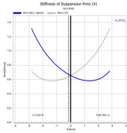
The stiffness  $K_{\rm ms}(x)$  which is the inverse of the compliance  $C_{\rm ms}(x)$  describes the ratio of the instantaneous force and displacement at the working point x. A steep increase of the stiffness indicates the limit of the moving capability of the mechanical suspension. A variation of  $K_{\rm ms}(x)$  corresponds with an instantaneous variation of the resonance frequency  $f_{\rm s}(x)$  and the mechanical loss factor  $Q_{\rm ms}(x)$  versus displacement.
