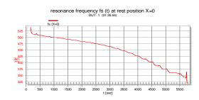
Reversible and nonreversible processes such as creep or ageing cause a decrease of the stiffness and resonance frequency during the measurement time which is normal for most drivers (figure below). A sudden decrease of
