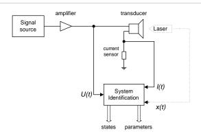
A laser sensor based on triangulation principle (see A2 Laser Displacement Sensor) can be used for measuring the voice coil displacement during the test. This information is used for identifying the force factor BI(x=0). This is required to calibrate the mechanical parameters in absolute terms.
