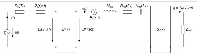
The lumped parameter model shown above is used to describe the large signal behavior of electro-dynamical drivers at high amplitudes. In contrast to the well-known linear model, most elements cannot be assumed to be constant but they depend on one or more speaker states (e.g. displacement x, voice coil velocity v, input current i, voice coil temperature  $T_v$ ):
