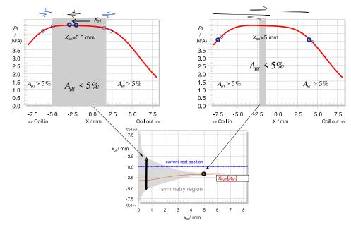
When operating a transducer in the small signal domain, where the amplitude AC signal is negligible, the symmetry point  $x_{sym}(x_{ac} \approx 0)$  is identical with the location at maximum force factor. However, the symmetry point  $x_{sym}(x_{ac} \approx x_{max})$  measured in the large signal domain where the amplitude is close to the maximum displacement  $x_{max}$  is more relevant for
