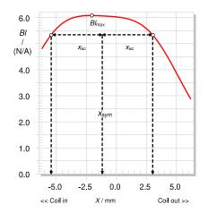
In general, the symmetry point  $x_{\text{sym}}(x_{\text{ac}})$  depends on the amplitude  $x_{\text{ac}}$  as shown as the red line in the lower diagram:
