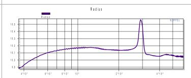
The *Result Table* window will return the effective radiation area and the equivalent radius averaged over your determined bandwidth. The window *Radius* shows the radius in terms of frequency. Ideally it would be a plane curve, but you may change your frequency bounds to select an almost plane area of the curve (in the example above between 70 and 250 Hz) and repeat your calculation to obtain a more exact solution.
