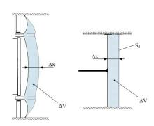
At sufficiently low frequencies every loudspeaker can ideally be represented as an infinitely rigid piston, which displaces the same air volume  $\Delta V$  at a constant voice coil displacement  $\Delta x$ . The area of this piston is always smaller than the real cone area and it is characterized as the effective radiation area  $S_{
