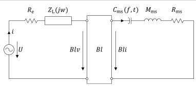
The moving mass  $M_{\rm ms}$  and the compliance  $C_{\rm ms}$  generate a vibrating system with a resonance frequency:
