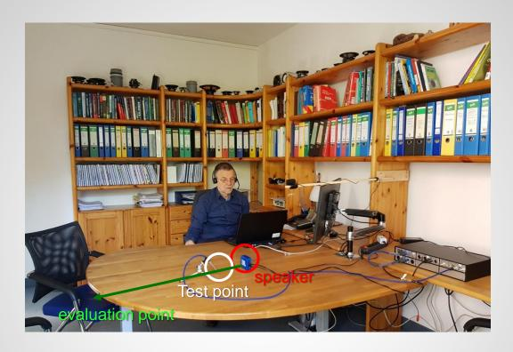
評估點1m距離處模擬自由場、遠場條件 Simulated Free-field, Far-field condition at evaluation point 1m distance
