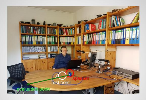
評估點1m距離處模擬自由場、遠場條件 Simulated Free-field, Far-field condition at evaluation point 1m distance
